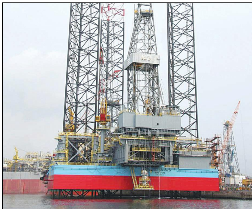
A jack-up drilling rig built at Jurong Shipyard in Singapore: funding availability makes newbuildings preferable to upgrading older units.
