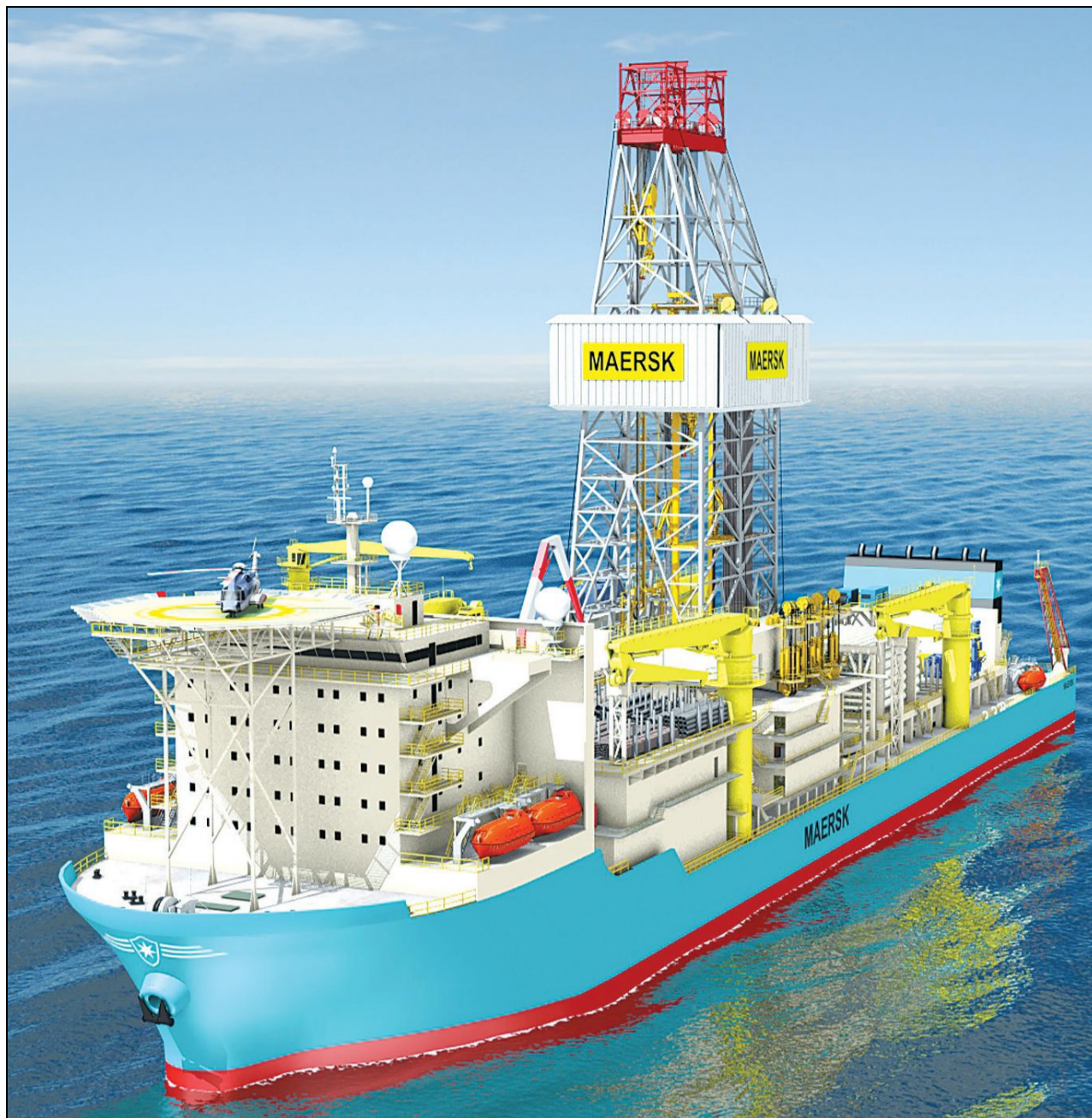
Maersk Drilling's two new drillships will be able to drill in water depths of 12,000 ft and be capable of drilling wells of more than 40,000 ft.
