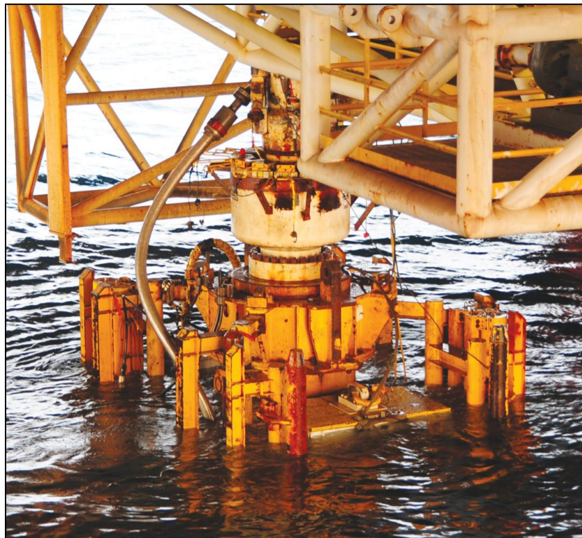
Attention is on redundancy in the blowout preventers on rigs, in the wake of last year's Macondo spill.
